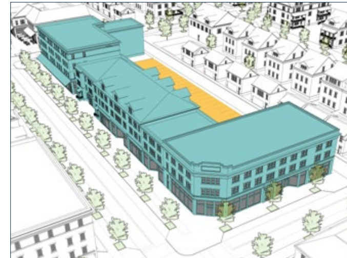
Building Orientation Illustration - Building is at the Street with Parking in the Rear.
